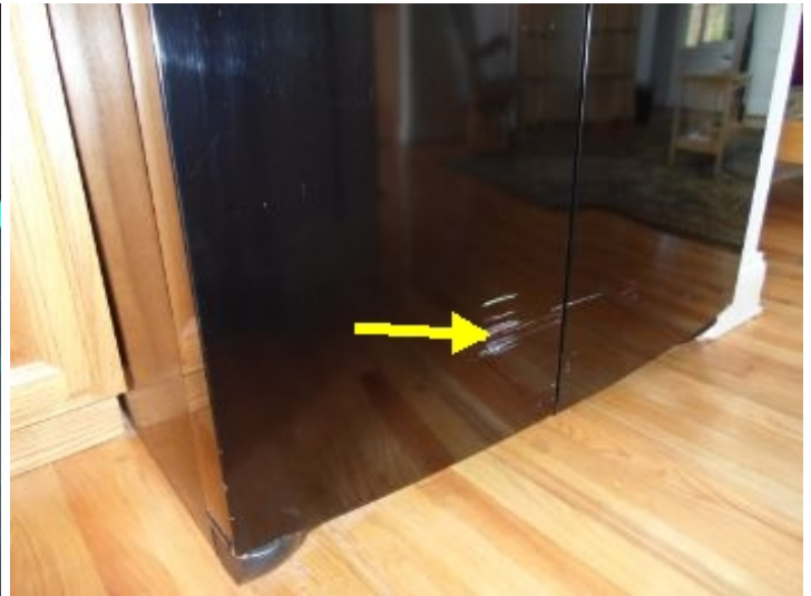
Damaged to the front of the fridge and the water and ice maker feature did not operate when tested.
